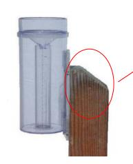
**Bevel** the top of the post to reduce rain splashing into the gauge.
