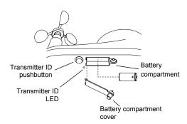
To verify power, wait 30 seconds then push and release the white transmitter ID pushbutton next to the battery compartment. The green transmitter ID LED next to the battery compartment will illuminate when you press the pushbutton.
