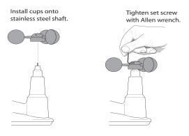
Note: If the wind cups don't spin freely, loosen the set screw, remove them from the shaft, and repeat the wind cup installation process.
